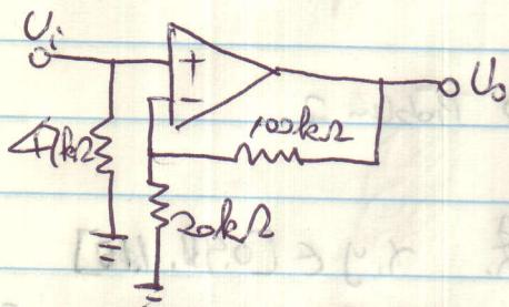
$$A = \frac{R_f + R_2}{R_1} = \frac{100 + 20}{20} = +6$$
