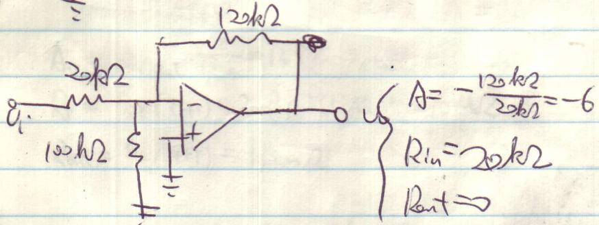
$$\left\{ \begin{array}{l} A = -\frac{120k\Omega}{20k\Omega} = -6 \\ R_{\text{in}} = 20k\Omega \\ R_{\text{out}} \Rightarrow \end{array} \right.$$
